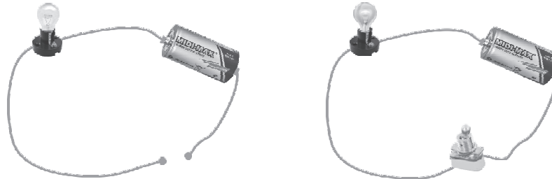
(a) Open circuit- the bulb does not glow and (b) Closed circuit the bulb lights up
